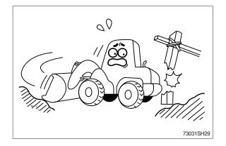
Always operate machine with proper ROPS/ FOPS installed.
