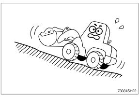
Operate the machine after making ground flat when operation is required on a slope.
